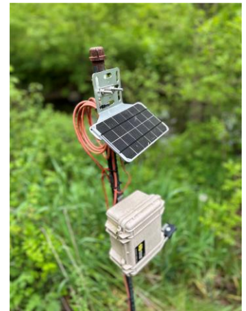
Solar-powered EnviroDIY Station on Dowagiac & Coldwater Rivers transmit real-time data to the web.
